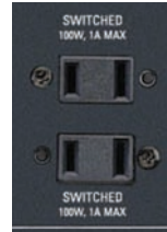
Figure 21 – Switched AC Accessory Outlets
